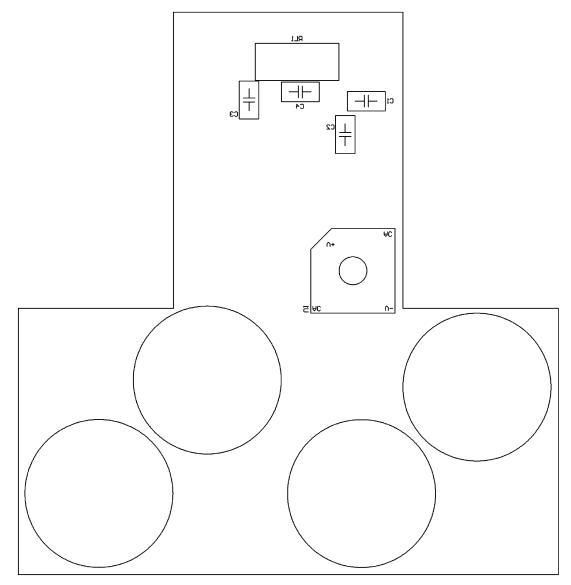
Figure 13. PCB Bottom Silkscreen View
