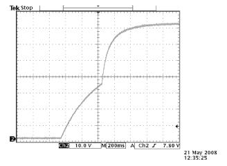
Figure 5. Supply Ramp at Power On
