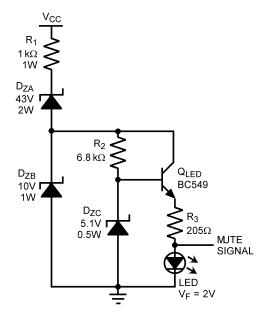
Figure 10. Constant Brightness LED and Mute Control Circuit
