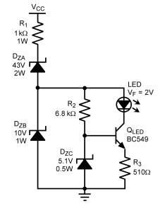
Figure 9. Constant Brightness LED Circuit
