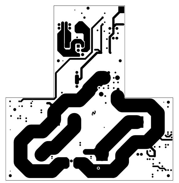
Figure 14. PCB Top Layer View
