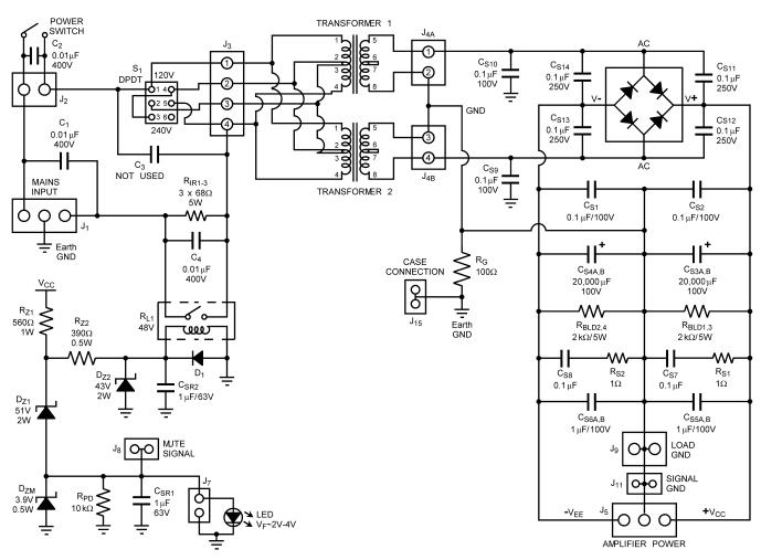
Figure 1. Complete Power Supply Circuit
